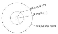
Figure 2.3.0a - Installing the External GPS Antenna (II)
